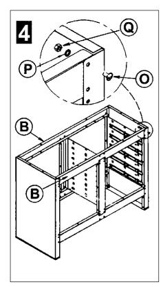
**STEP 4.** Take two crossrails (B) and bolt them to the cabinet sides (A) and centre supports (C) using 12 bolts (O), 12 lock washers (P), and 12 nuts (Q).
