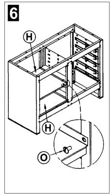
**STEP 6.** Bolt the two shelf components (H) into position in the left hand compartment using 8 bolts (O), 8 lock washers(P), and 8 nuts (Q).
