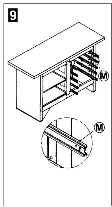
STEP 9. Take the 10 male slide components (M) and slide 5 onto the female slides on the left of the draw compartment and 5 onto the female slides on the right hand side of the draw compartment. Push them fully in to engage them, then pull them out to the stop point.
