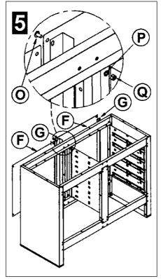
STEP 5. Take the two draw stops (G) and one back panel (F) and bolt them to the back of the cabinet with the draw stops between the panel and the cabinet. Bolt the other back wall panel into position using bolts (O), lock washers (P), and nuts (Q).
