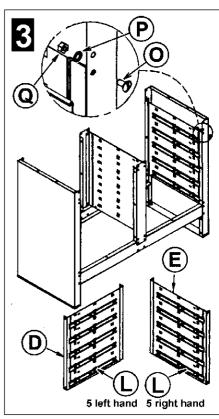
STEP 3. Bolt left & right slide panels (D) & (E) into position using 8 bolts (O), 8 lock washers (P), and 8 nuts (Q). Fix 5 left hand female slides (L), onto slide panel (D) and 5 right hand female slides (L), onto slide panel (E)
