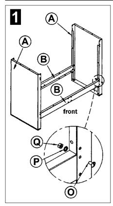
STEP 1. Take two crossrails (B) and bolt them to the cabinet sides (A) using 8 bolts (O), 8 lock washers(P), and 8 nuts (Q). Ensure that the pairs of holes that accept the corner braces are facing downwards. ( Refer to STEP 7.)
