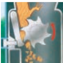
Adjustable drum – material is shredded by a combined crushing and cutting process.
