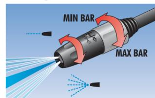
The spray angle of the nozzle can be adjusted from a wide fan to a jet. Various pressure settings can also be set steplessly: the high-pressure setting for fast, powerful cleaning, and the low-pressure setting for gentle cleaning.
