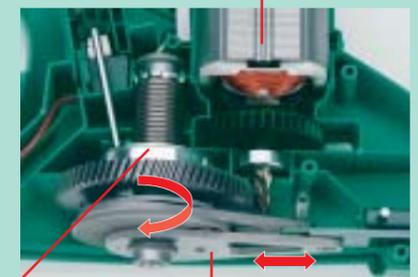
Slipping clutch (extremely high torque: 80 Nm)
