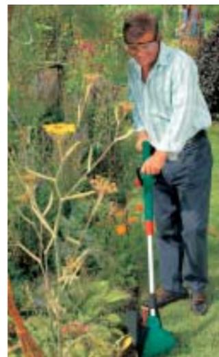
For cutting along edges and borders, the trimmer head can be turned 90 degrees from the horizontal position into a vertical position. This ensures that the gardener always has a clear view of the cutting edge while walking forwards and can easily cut the edges straight. The fold down plant protector ensures trimmer line is kept at a safe distance to protect border plants and tree trunks.
