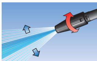
The jet-fan nozzle delivers constant pressure and can be adjusted from a wide fan spray to a single jet. Use the fan spray for cleaning large surface areas. Stubborn dirt can be removed with the more powerful jet.
