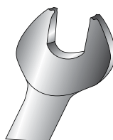
Never work with damaged or chipped tools
