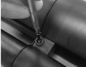
Insert both tubes into the main body and screw together with the large screw.
