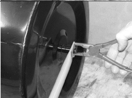
Secure with the E-Clips and Washers supplied. The E-Clips will need to be squeezed onto the Roller Shaft using pliers
