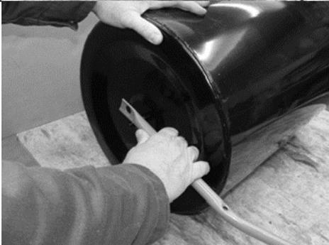
Then pull the other end of the Handle to place it over the other end of the Roller Shaft. You may need to bend the Handle slightly to stretch it over the Roller Shaft.
