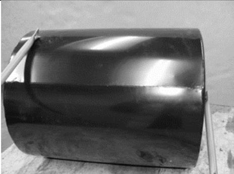
Fit the Lower Handle to the Roller by placing one end of the Handle over the Roller Shaft.
