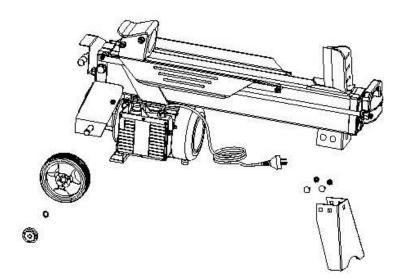
2. Carefully fit the log splitter to your fully assembled stand, use the nuts and bolts supplied (part list items 5&6) to secure the log splitter to the stand. See figure 4.
