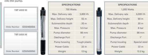
Deep well / Bore hole pumps suitable for great depths. With an integrated check valve so water cannot flow back into the pump.
