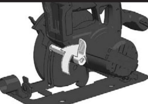
Adjust the cutting depth to the thickness of the workpiece. Less than a full tooth of the blade teeth should be visible below the workpiece.
