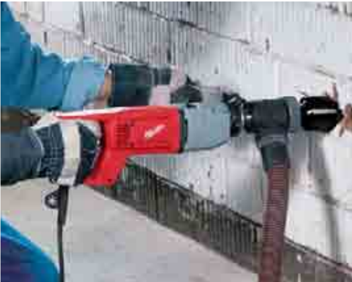
Picture shows optional accessory. FIXTEC Clean Line Rotor for drilling in dust extraction.
