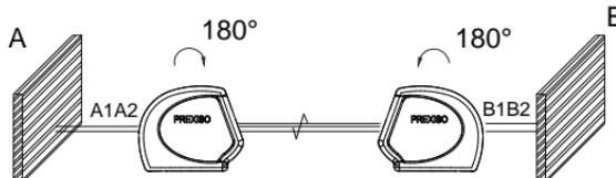
Turn on the cross line laser to horizontal leveling in unlocked mode. Set the instrument on a leveling half-way between two walls (A+B).
