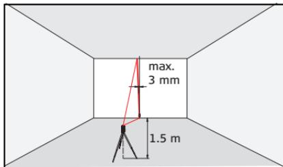
As reference, use a plumb-bob and attach it as close as possible to an approx. 3 m high wall.
