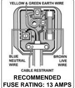
Double insulated products, which are always marked with this symbol , are fitted with live (brown) and neutral (blue) wires only. To rewire, connect the wires as indicated in diagram. **DO NOT** connect either wire to the earth terminal.
