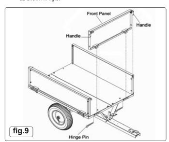
5.8.3 Lock each side panel to the front panel as follows. Rotate the handles at each top corner of the front panel (see fig.9) through 180° so that they are pointing upwards. Let the bent part of each handle protrude into the slotted tag on each side panel. Rotate the handles back down into their original positions so that the slotted tags are retained against the side edges of the front panel.
