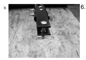
Insert the Towing Pin and secure with the R-Clip, as shown.
