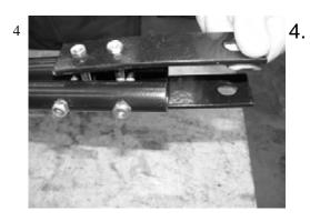
Fit the two Clevis Jaws to the Drawbar using two 55mm Bolts and Nuts, ensuring that the Bolts are between the two front 70mm Bolts and the two Drawbar parts, as shown.
