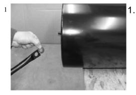
. Insert a Plastic Bush onto the inside of the Drawbar.
