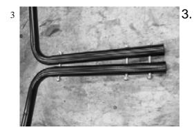
Loosely fit the three 70mm Bolts and Nuts through both parts of the Drawbar, as shown.
