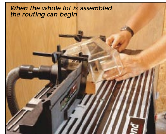
The extractor pipe plugs into the back of the fence using the adaptor kit
