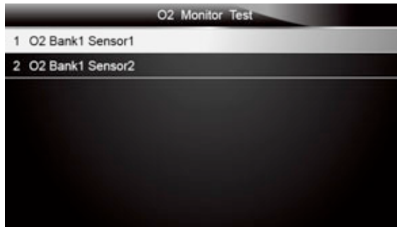
Figure 5-24 Sample O 2 Monitor Test screen
