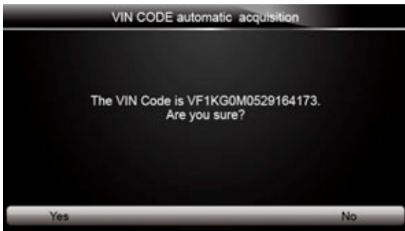
Figure 4-5 Sample VIN Automatic Acquisition
