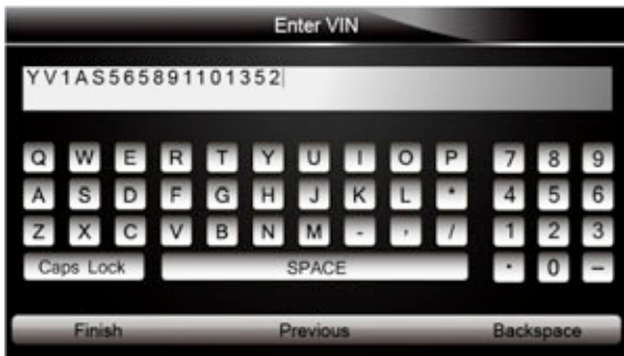
Figure 4-7 Sample Manual VIN Entry with Keyboard
