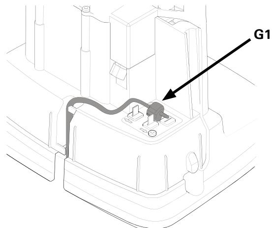
Connect the guide wire to the charging station as follows:
