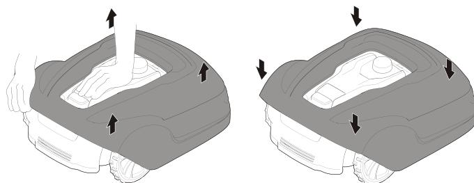
Hold down the mower with one hand and lift firmly at one of the corners of the body and repeat for all four corners, until the body pops loose from the chassis.
