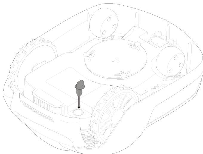
Insert the safety key into the underside of mower and turn to the **Enable** position.
