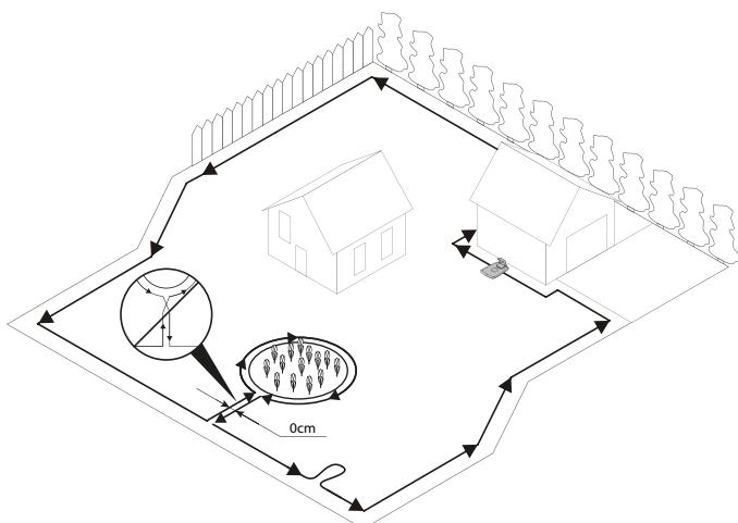
Temporarily secure the end of the loop wire to a peg or other object at the charging station.
