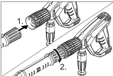
→ Insert the high pressure nozzle onto the spray lance.
