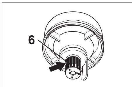
The suction canal (6) is equipped with a float.
