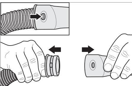
The suction hose is equipped with a clip system. All C-35/C-DN-35 accessories can be connected.
