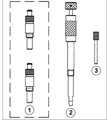
1 VS4926 Camshaft setting pins (pair)
